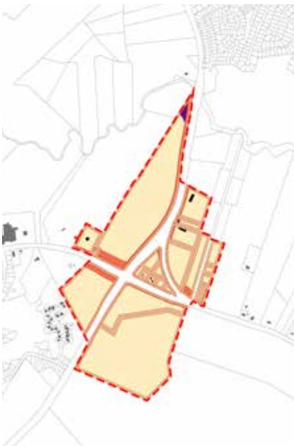
Combined Buffers and Setback Constraints The diagram above shows all of the buffers that impact the District 5 properties, in addition to the 50-foot setbacks from all property lines.
