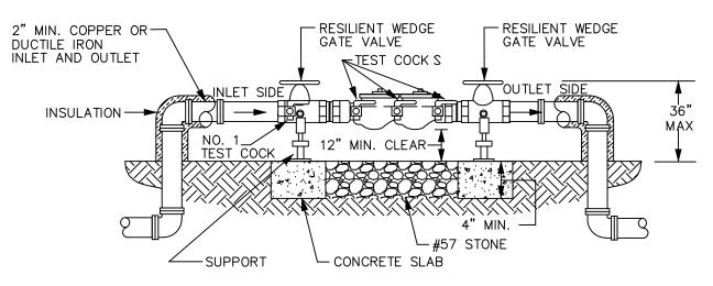
NOTE: APPROPRIATE THRUST RESTRAINT AND SUPPORT MEASURES ARE TO BE PROVIDED.
